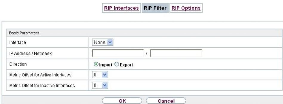
Fig. 122: Routing Protocols->RIP->RIP Filter->New
