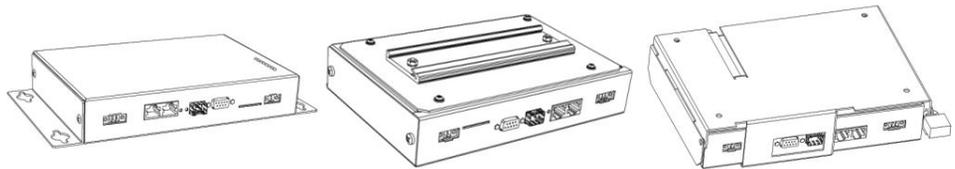
Fig. 12: Wall mounting of the **bintec Wix040n** (standard design, DIN rail or theft protection optional)
