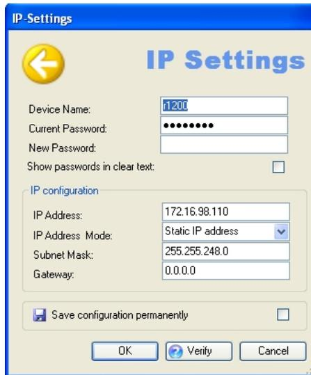
Fig. 29: IP address assignment with the **Dime Manager**
