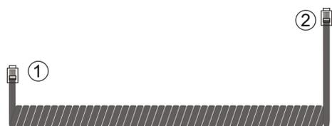
Insert the RJ11 plug ① into the RJ11 socket on the receiver.
