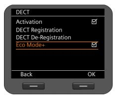
If the function is activated, **Eco Mode+** is highlighted with  $\mathbf{M}$ .
