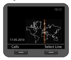
When setting the **Time Zones**, a map of the world showing the time zones appears on the screen. The current setting is highlighted.
