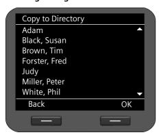
If it is not possible to view all of the functions/ list entries at the same time (list is too long), arrows appear on the right-hand side. The arrows indicate the direction in which you need to scroll to view the rest of the entries in the list.
