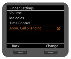
If the function is activated, the **Anon. Call Silencing** entry is marked with  $\[ \]$  . The phone will then not ring if an anonymous call is received. The call is still shown on the display.
