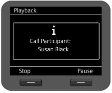
The name of the participant will be displayed during playback. The elapsed time and the total duration of the call record are displayed in the top right corner.
