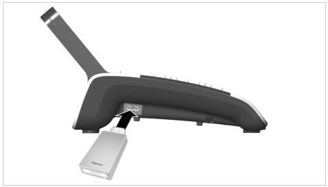
▶ Connect the USB stick to the USB port on the device.
