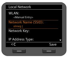
It is possible to avoid sending the SSID and therefore hide the WLAN. Such WLANs cannot be found during a network search. If the WLAN that you want to connect to prevents the SSID from being sent, you will have to connect manually.
