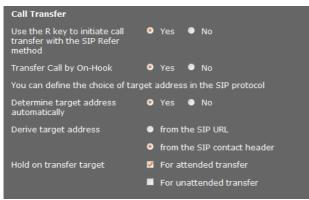
Participants can transfer a call to another participant as long as the PABX/provider supports this function. The call is transferred using the handset menu (via the display key) or using the R key (+ page 35).
