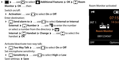
The destination number is displayed in idle display when the room monitor is activated.
