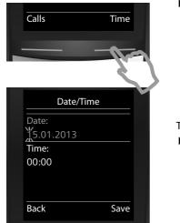
Press the key Time below the display screen to open the input field.
