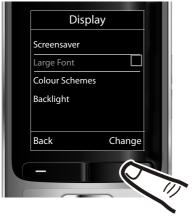
▶ Press down on the control key until the Large Font menu option appears on the display.
