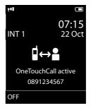
By pressing any key the saved number is dialled. Press the end call key , to cancel the dialling operation or to end the call.
