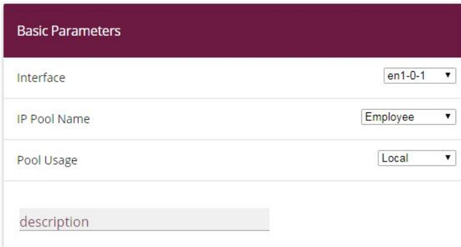
The screenshot shows a web interface for configuring a new DHCP pool. The title is "Basic Parameters". There are three dropdown menus: "Interface" set to "en1-0-1", "IP Pool Name" set to "Employee", and "Pool Usage" set to "Local". Below these is a text input field labeled "description" which is currently empty.
