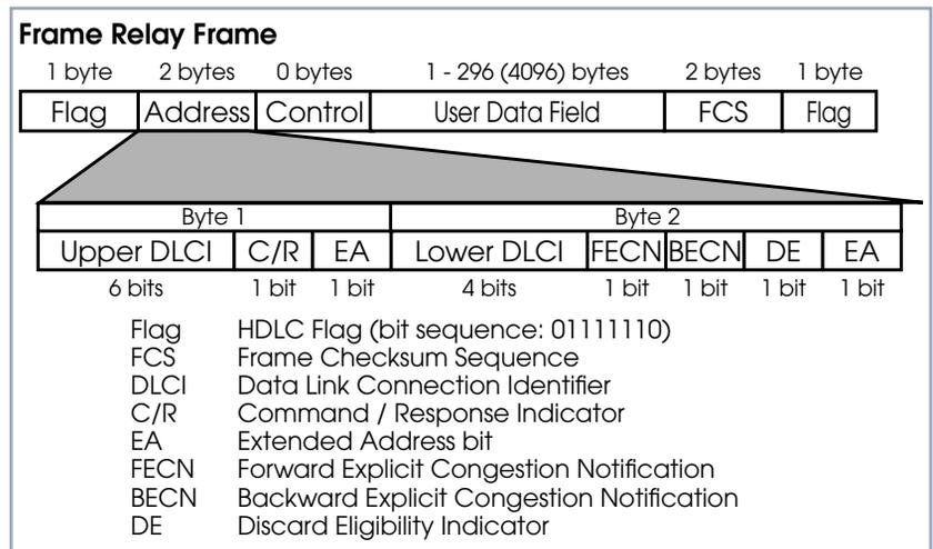
Figure A-3: Frame Relay Frame
