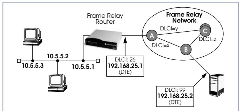
Figure A-5: Scenario: Frame Relay over ISDN Lines
