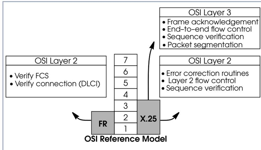
Figure A-2: Frame Relay in OSI Reference Model
