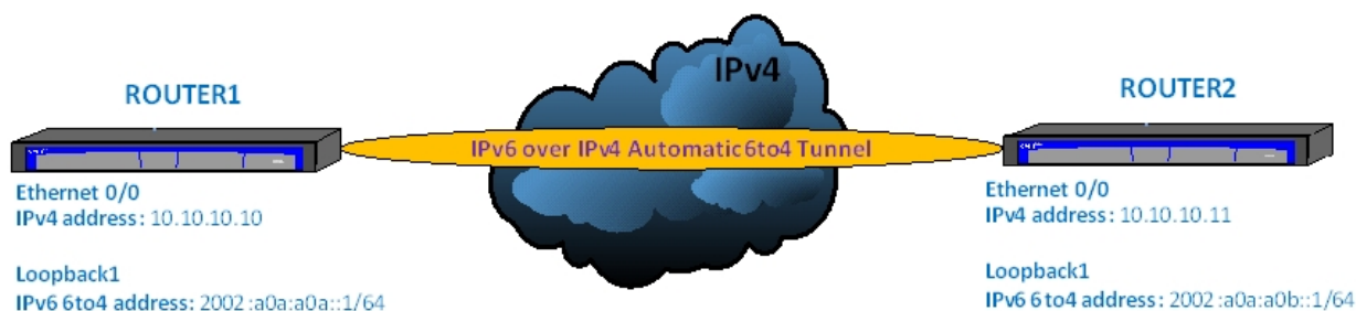
Fig. 5: Automatic 6to4 tunnel.
