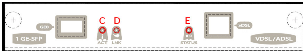
Fig. 3: TBC1-1VDSL1SFP card : LEDs.
