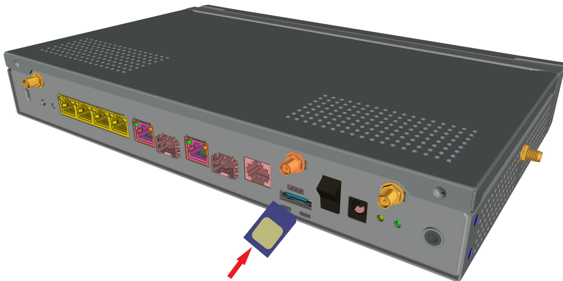
Fig. 21: Press to insert the SIM card into the tray
