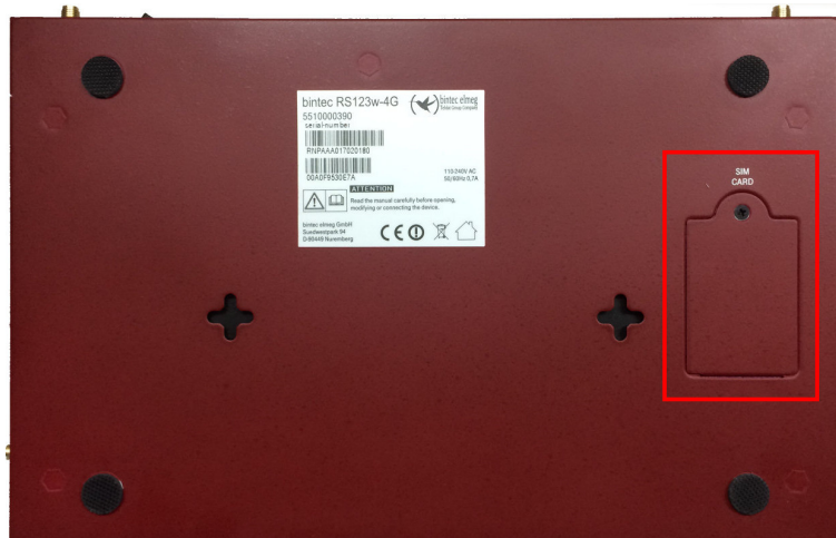
Fig. 16: Internal module SIM tray
