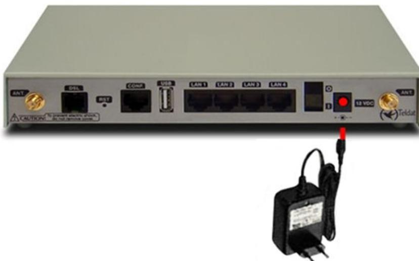
Fig. 4: Connecting the power with an external source
