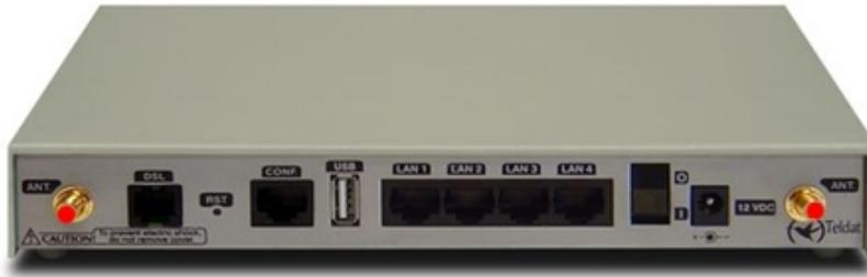
Fig. 9: Wireless LAN antenna connectors
