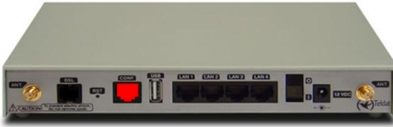
Fig. 11: Configuration connector
