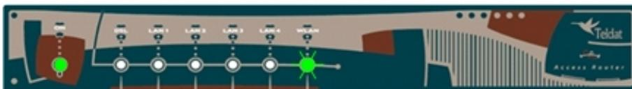
Fig. 15: Once the WLAN LED is blinking you can release the pushbutton
