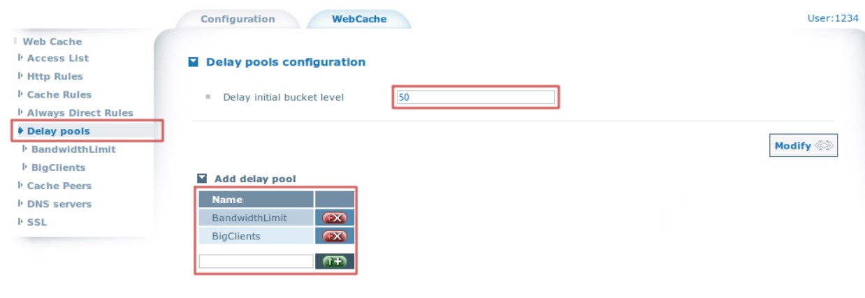
Fig. 3.15. Delay pools main configuration
