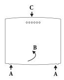
Opening the PABX: »C« is the front of the PABX system. Pull the two plastic springs marked »A« outward until the cover is released. Lift off the cover carefully toward the rear. It can then be easily lifted off. The terminal panel is then visible under the enclosure cover.
