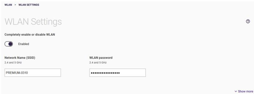
In the **WLAN settings** menu, you make the basic settings for operating wireless networks in the 2.4 and 5GHz bands. In the default settings, the WLAN is enabled and provides the same network in both frequency bands. If you have not yet made any changes here, you can change the network name or disable the WLAN completely.
