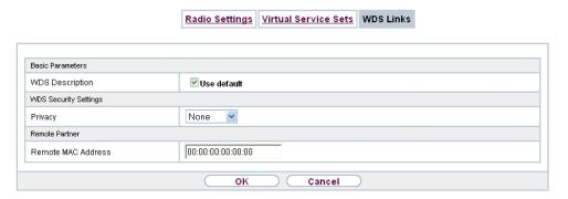
Fig. 73: Wireless LAN->WLAN->WDS Links->New
