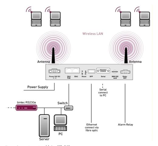
Fig. 11: Connection options bintec Wlx040n
