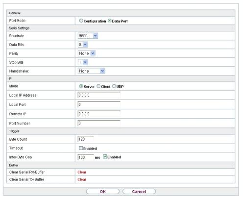
Fig. 61: Physical Interfaces->Serial Port->Serial Port with Port Mode = Data Port
