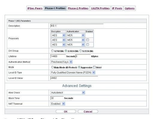
Fig. 142: VPN->IPSec->Phase-1 Profiles->New
