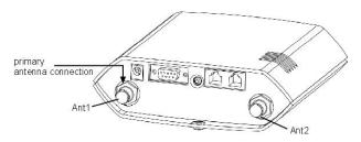
Fig. 81: Antenna connection
