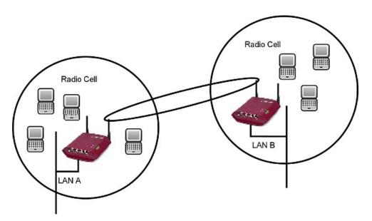
Fig. 79: Wireless bridge with connection of wireless clients
