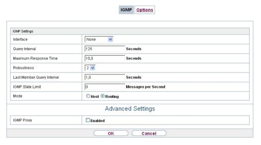
Fig. 125: Multicast->IGMP->IGMP->New
