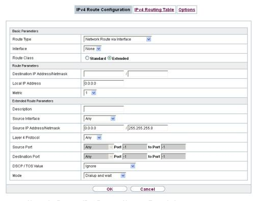
Fig. 101: Network->Routes->IPv4 Routes->New with Extended = Enabled
