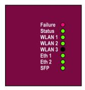
Fig. 15: LEDs of bintec WI1040n and bintec WI2040n
