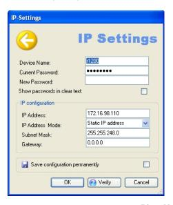
Fig. 29: IP address assignment with the Dime Manager
