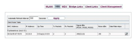
Fig. 208: Monitoring->WLAN->VSS
