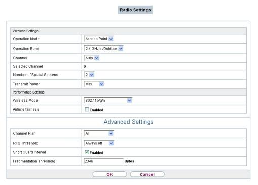
Fig. 69: Wireless LAN->WLAN->Radio Settings-> for Operation Mode Access Point
