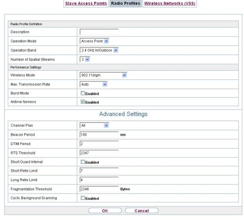
Fig. 89: Wireless LAN Controller->Slave AP configuration->Radio Profiles-> / New
