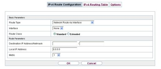
Fig. 100: Network->Routes->IPv4 Routes->New with Extended Route = Standard.
