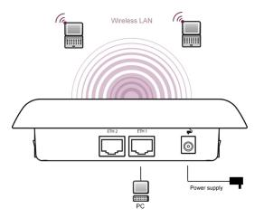
Fig. 2: Connection options bintec W2003n, bintec W2003n-ext, bintec W2004n
