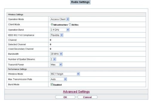
Fig. 70: Wireless LAN WLAN Radio Settings for Operation Mode Access Client The Wireless LAN->WLAN->Radio Settings-> menu consists of the following fields:
