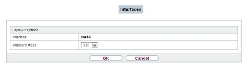
Fig. 46: System Management->Interface Mode / Bridge Groups->Interfaces->Add You can realise bridging for devices behind access clients with the MAC Bridge function. In wildcard mode you cannot define how Unicast non-IP frames or non-ARP frames are processed. To use the MAC bridge function, you must carry out configuration steps in several menus.
