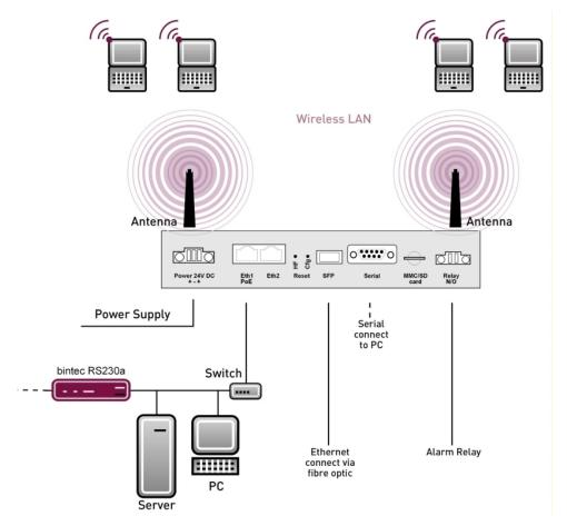
Fig. 18: Connection options bintec Wlx065n
