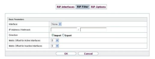
Fig. 122: Routing Protocols->RIP->RIP Filter->New
