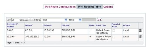
Fig. 102: Network->Routes+IPv4 Routing Table
