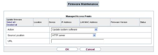
Fig. 87: Wireless LAN Controller->Maintenance->Firmware Maintenance
