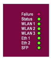
Fig. 13: LEDs of bintec WI1040n and bintec WI2040n
