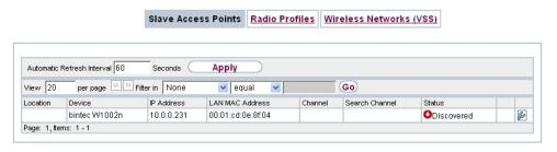
Fig. 78: Wireless LAN Controller->Slave AP configuration->Slave Access Points
