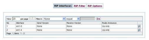
Fig. 106: Routing Protocols->RIP->RIP Interfaces
