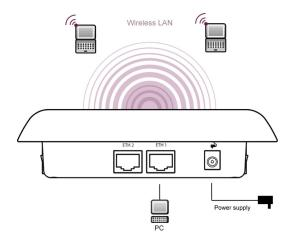
Fig. 2: Connection options bintec W2003n, bintec W2003n-ext, bintec W2004n
