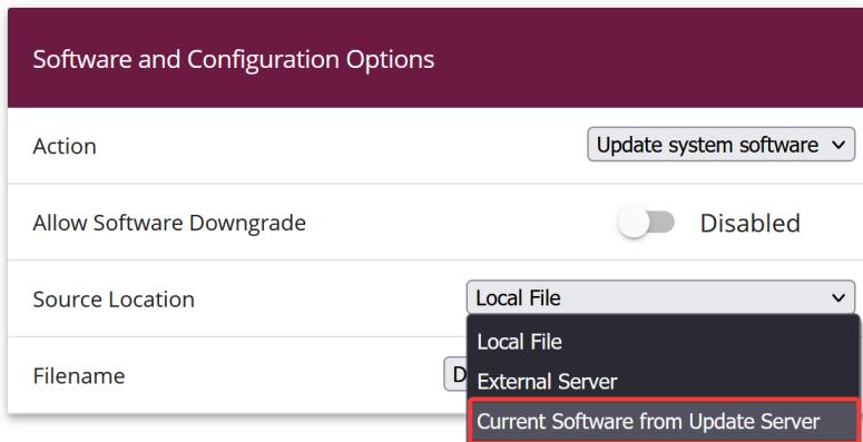
If your access point does not yet have internet access, you can also download the software image from our server (<https://archive.bintec-elmeg.com/?dir=Files/WLAN/IMG-Series>) and then carry out the update by choosing the option **Local File** for the **Source Location**.
