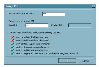
The PIN for a Smart Card or for a soft certificate can be changed under the menu item "Change PIN", if the correct PIN number has previously been entered. This menu item will not be activated without the previous entry of a valid PIN number.
