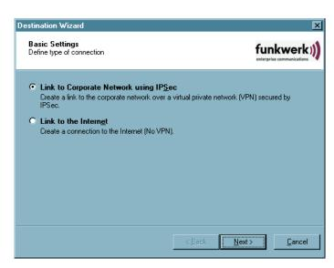
Using the configuration assistant, connections can be quickly established with the Internet or to the corporate network. The profile is created after a few configuration questions, in accordance with the selection of the desired basic setting.
