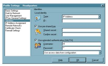
If you use Extended Authentication, User Name and Password must be entered in the configuration folder of the profile. Otherwise the establishing of a connection will not be successful (see → Profile Settings, Identities, Use extended authentication (XAUTH)).
