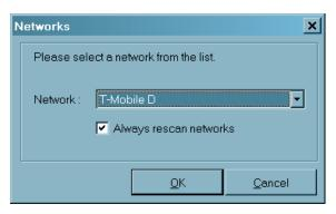
If a network search was executed. the window for network selection will be displayed (left). The desired network can be selected from a list. If you do not desire another network search each time the Monitor is called, is then this function, which is active by default, must be switched off via the Check button.
