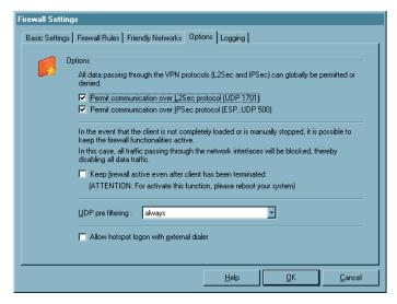
With blocked basic setting the set-up of VPN connections via the "Options" tab can be globally permitted. The following protocols and ports required for the tunnel set-up are released per generated filter:
