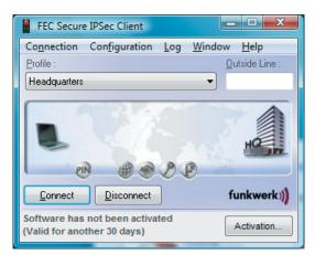
The time remaining until software activation, i.e. the validity period of the test version, is displayed in the message bar of the monitor next to the activation button.
