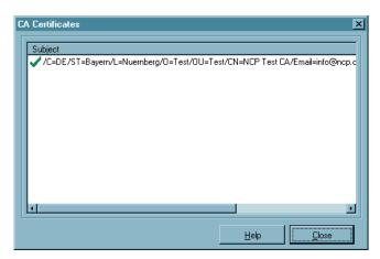
Multiple issuer certificates are supported with the client software (multiple CA support). The issuer certificates must be collected in the installation directory under CACERTS\ for this. In the client monitor the list of CA certificates read in is displayed under the menu item "Connection → Certificates → Display CA Certificates",
