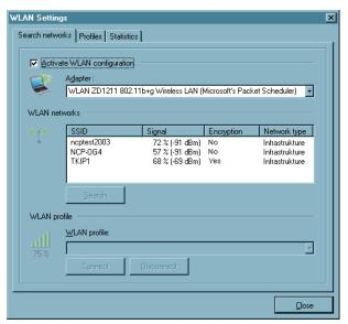
If this "WLAN Configuration" is activated, then the management tool of the WLAN card must be deactivated. (Alternatively the management tool of the WLAN card can also be used; in this case the WLAN configuration in the monitor menu must be deactivated.)
