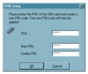
After three incorrect attempts to enter the SIM PIN the window for entering the PUK (Personal Unblocking Key), which accompanies the SIM card, will be displayed. After correctly entering the PUK you will be able to enter a new SIM PIN.
