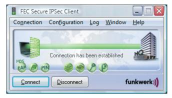
It is also possible to manually establish the connection to a selected destination by selecting "Connection" in the main menu and click on "connect" Alternatively you can click on the "connect" button in the tool bar.
