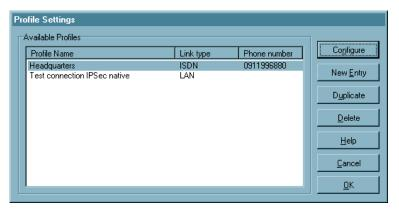
The buttons located to the right can be used to add, remove, copy and modify the entries of the profiles.
