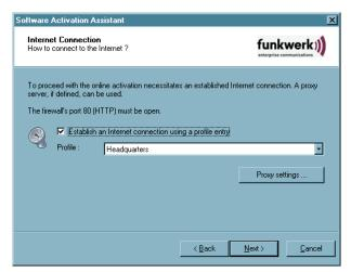
If the IPSec Client is used to set-up the connection on the Internet, then a suitable profile must first be established for the IPSec Client. Ensure in this regard that port 80 is released (for HTTP) if the firewall is activated. (If a proxy server will be configured in the operating system, then these settings can be transferred.)
