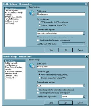
In this regard ensure that the destination system with automatic media detection is configured with all parameters necessary for the connection to the VPN Gateway (particularly the IP address of the VPN gateway), on the other hand the destination systems with the alternative connection types must be configured in such a manner that each desired connection type (possibly the modem parameters as well) is set and the function "Entry for automatic media detection" is activated.
