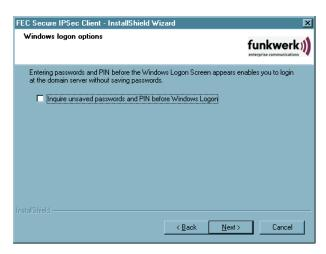
Thereafter you can define whether a logon to a remote domain should occur after establishing a connection to the remote destination's NAS, which may necessitate entering the PIN for your certificate and/or your Password (if not already stored in the Client Software). After establishing a connection to the remote destination's NAS, you can logon to the remote domain. This logon will be encrypted.
