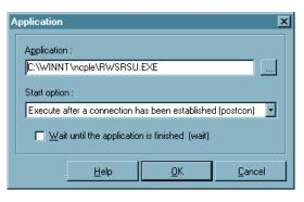
Use this configuration to start applications or batch files, depending on the Client Monitor. The external applications are added as described below. The sequence, in which they are called, from top to bottom, can be changed with the green arrow keys.
