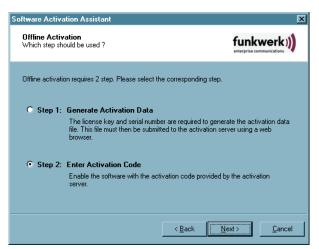
The second step of the offline variant is triggered via the Monitor menu "Help" "License info and activation". After the offline variant has been selected, select the second step.
