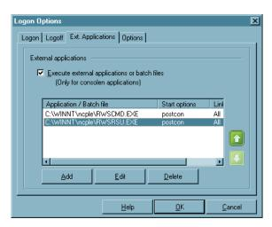
Use this configuration field to start applications or batch files, depending on the Client Monitor (no Windows programs!).
