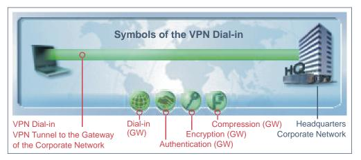
The colors of the icons change from gray to black, then flash green, and finally are displayed as constant green to indicate successful connection set up. In this regard the dial-in and authentication processes on the gateway must always be executed; encryption and compression are optional. From left to right the VPN dial-in icons are:
