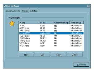
Previously created profiles for the adapter selected above are displayed in a list. Network type, encryption, and SSID must agree with the above network parameters. A new profile is generated by clicking on the "New" button, or by double clicking on the corresponding network in the previous window, or by clicking on the right mouse button. Profiles can also be edited or deleted via the buttons.
