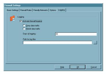
The activities of the firewall are written to log file depending on the setting. The default location of the "Output directory for log files" is in the installation directory under \log.
