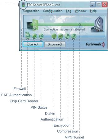
In addition either WLAN panel or a UMTS / GPRS panel will be displayed in the monitor depending on configuration and installation of a multifunction card.
