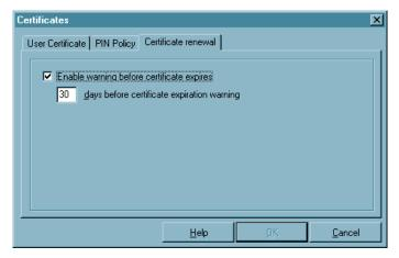
In this configuration field you can specify whether a message is given out that warns of the expiration of validity, and you can specify how many days before the certificate validity expiration this message should go out. As soon as the set time frame before expiration goes into effect, a message will appear each time a certificate is used, indicating the expiration date of the certificate.
