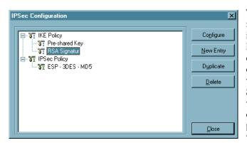
This menu item is clicked for configuring policies and, if necessary, a static Secure Policy Database. A configuration window will open displaying the branch with the policies and the Secure Policy Database as well as buttons for operation in the right-hand part of the configuration window.
