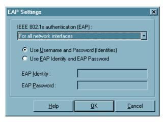
You can specify whether EAP authentication will only be executed via WLAN cards, LAN cards, or via all network cards, in the "EAP Options" of the Monitor menu. The setting made here applies globally for all phonebook entries. In an activation box the EAP authentication can be set as follows:
