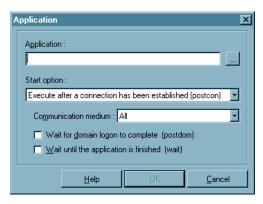
After you have selected the function "Start external applications or batch file" you can select an application or batch file from the computer (see previous page), this application of batch file is then loaded depending on the start option:
