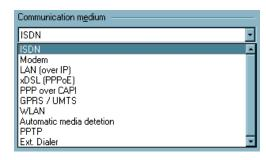
You can select the communication medium for each profile, provided that you have the required device installed on your PC and recognized by Windows.
