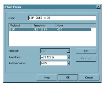
The parameters in this field relate to phase 1 of the Internet Key Exchange (IKE) with which the control channel for the SA negotiation was established. You determine the IKE mode (Exchange Mode), main mode or aggressive mode, in the Phonebook under "IPSec General Settings".
