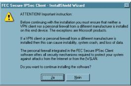
Note the following message and deactivate any VPN Client and Personal Firwall of another manufacturer to avoid data loss.
