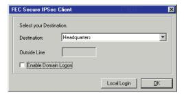
To initiate a link to be built, select the destination system to connect to and then click on the OK button.
