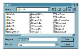
Clicking this button will open a window where you can enter the name and path of the file to be created for the log feature to write (record) to (default name = ncptrace.log).
