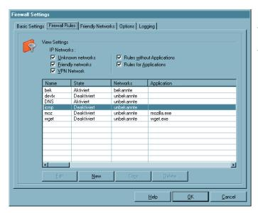
The rules for the extended firewall are brought together in this configuration field. The display options are all active by default and correspond to the selected networks, for which the respective rule can be defined, and whether this rule will be valid regardless of application:
