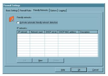
If in "Firewall rules" you have defined in the configuration field, that a rule will be applied to connections with known network, then this rule is always used, if a network can be identified as known network according to the criteria that is entered here, e.g. the LAN adapter is in a known network.
