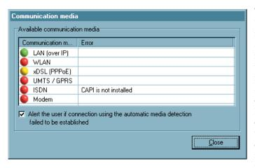
The purpose of this window is only to inform about the available communication media and the currently used communication medium. On the basis of a pre-configured destination system, those link types that are currently available for the Client PC are detected and implemented, and if multiple alternative transmission paths are available, the fastest will be selected automatically.
