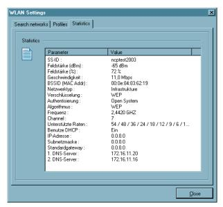
The statistics window for the WLAN settings shows the status of the connection to the Access Point in plain text.
