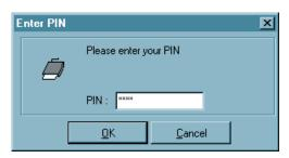
If the PIN has not been entered before a connection establishment, then the PIN entry dialog appears when the first connection requiring the use of a certificate is to be established to a destination at the latest. Thereafter the PIN entry can be comitted in the case of repeated manual connection establishment, if this has been configured (see →Configuration, Certificates).
