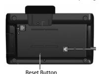
The reset button is located behind the small opening labelled **Reset**. Use a pointed item, e.g., a paper clip.
