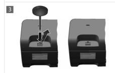
Remove the handset retainer from the cradle using the tool provided, and replace it with the ridge pointing upwards.
