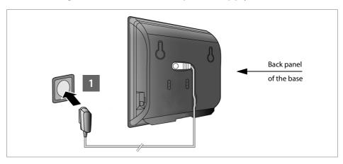
1 Insert the power adapter into the mains socket.
