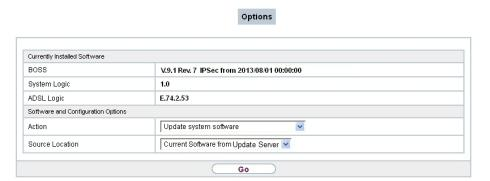
The device will now connect to the bintec elmeg GmbH download server and check whether an updated version of the system software is available. If so, your device will be updated automatically. When installation of the new software is complete, you will be invited to restart the device.
