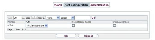
Fig. 70: LAN->VLANs->Port Configuration
