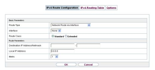
Fig. 81: Network->Routes->IPv4 Route Configuration->New with Extended Route = Standard.
