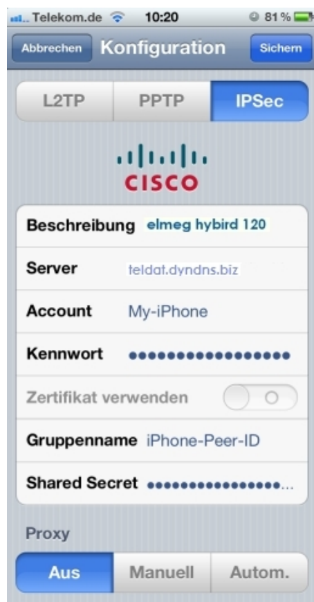
Fig. 163: Settings -> General -> Network -> VPN -> Add VPN Configuration
