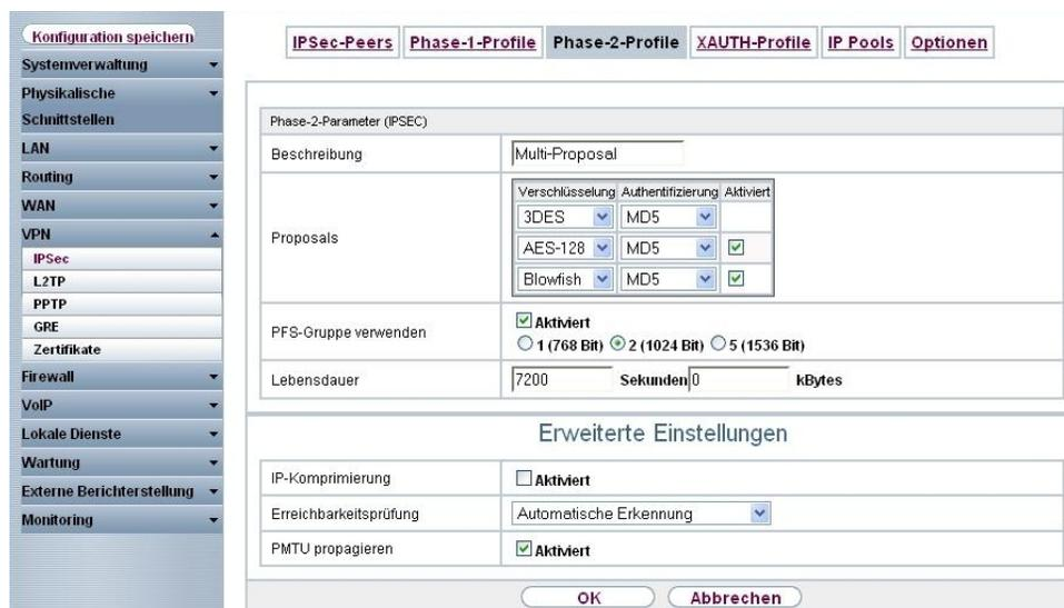
The screenshot shows the configuration interface for Phase-2-Profile. On the left is a navigation menu with categories like Systemverwaltung, Physikalische, and VPN. The main area has tabs for IPsec-Peers, Phase-1-Profil, Phase-2-Profil, XAUTH-Profil, IP Pools, and Optionen. The Phase-2-Profile configuration includes:
