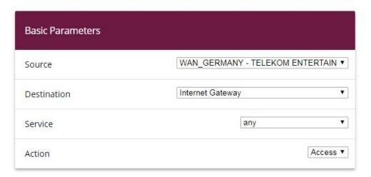
Fig. 41: Firewall->Policies->IPv4 Filter Rules->New
