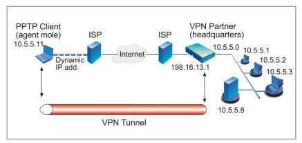
Figure B-3: A typical client-to-LAN scenario.
