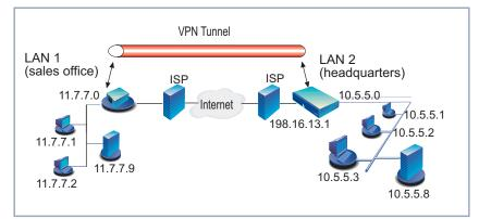
Figure B-1: Example LAN-to-LAN configuration
