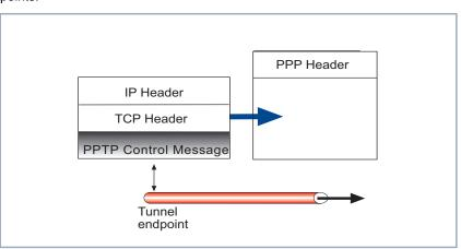
Figure A-2: Tunnel establishment phase
