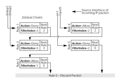
The diagram below shows in detail how Access List, Rules and Filters are applied to incoming IP traffic.
