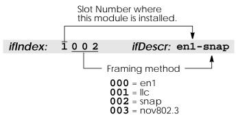
The *ifIndex* shown above identifies a point-to-multipoint interface installed in slot 1. On most systems this is the CM-BNCTP ethernet module but may also be a token ring module (CM-TR). The *biboAdmBoardTable* entries would verify this module. This hardware interface uses SNAP framing. For information on the frame formats used with point-to-multipoint interfaces refer to <u>Appendix B</u>).
