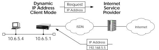
Upon receiving an IP address from the dialup (server) host, the BRICK will automatically create an IP route to allow hosts on the LAN to access networks via the dialup connection. The route is also automatically removed when the connection is closed. CAPI
