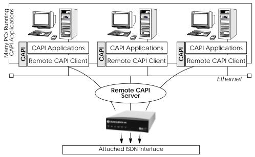
This Remote CAPI is a DualMode server, and supports version 1.1 and 2.0 CAPI. Each PC running Remote CAPI Client software can access the BRICK's ISDN interfaces as if the interfaces were available locally. To CAPI applications, messaging between client and server remains transparent.
