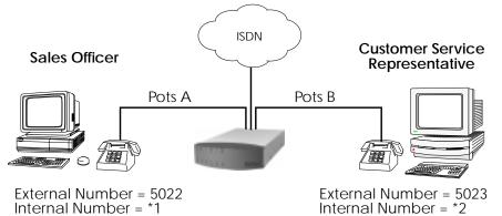
In the simple scenario shown above, the BRICK is used to make inter-office (toll-free) calls between workstations using the internal telephone numbers. In addition, both parties can simultaneously place or receive calls from the ISDN using their respective analog devices.
