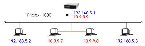
The ethernet interface for the BRICK in the diagram (assumed to already be assigned 192.168.5.1) could be assigned a second address by adding the following IP route.
