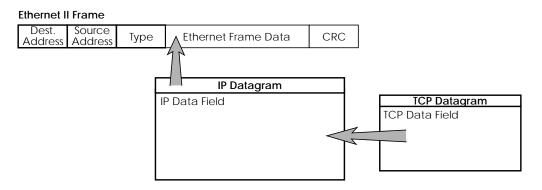
When filtering packets based on contents of the ethernet frame it's important to know the relative locations (offset) and possible values of the frame's fields. Below is
