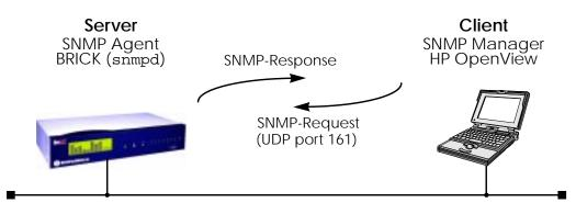
SNMP can be seen as a simple asynchronous **request-response** protocol. Messages are passed via UDP (normally port 161) and are binary in format. The SNMP Manager requests information from a specific device and an SNMP Agent (running on the device) authenticates the requester and responds with the requested information.
