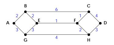
In OSPF each link has a cost associated with it (typically some fixed number divided by the bandwidth of the link). Routes are calculated and selected according to the least cost of the overall path a packet will travel. Thus in shortest-path routing the best path is also the fastest path (theoretically), regardless of the number of stations a packet travels through.
