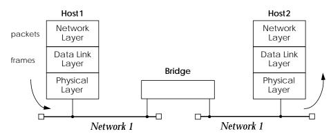
In transparent bridging each bridge makes its own routing decisions and is therefore 'transparent' to the communicating hosts on the end networks. Additionally, a transparent bridge configures itself (in terms of routing information) after coming into service.
