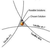
The current location could be any point within the gray-colored area. Precision is said to be *diluted* when the area grows larger. The monitoring and control of *dilution of precision* (DOP) is the key to writing high-precision applications.
