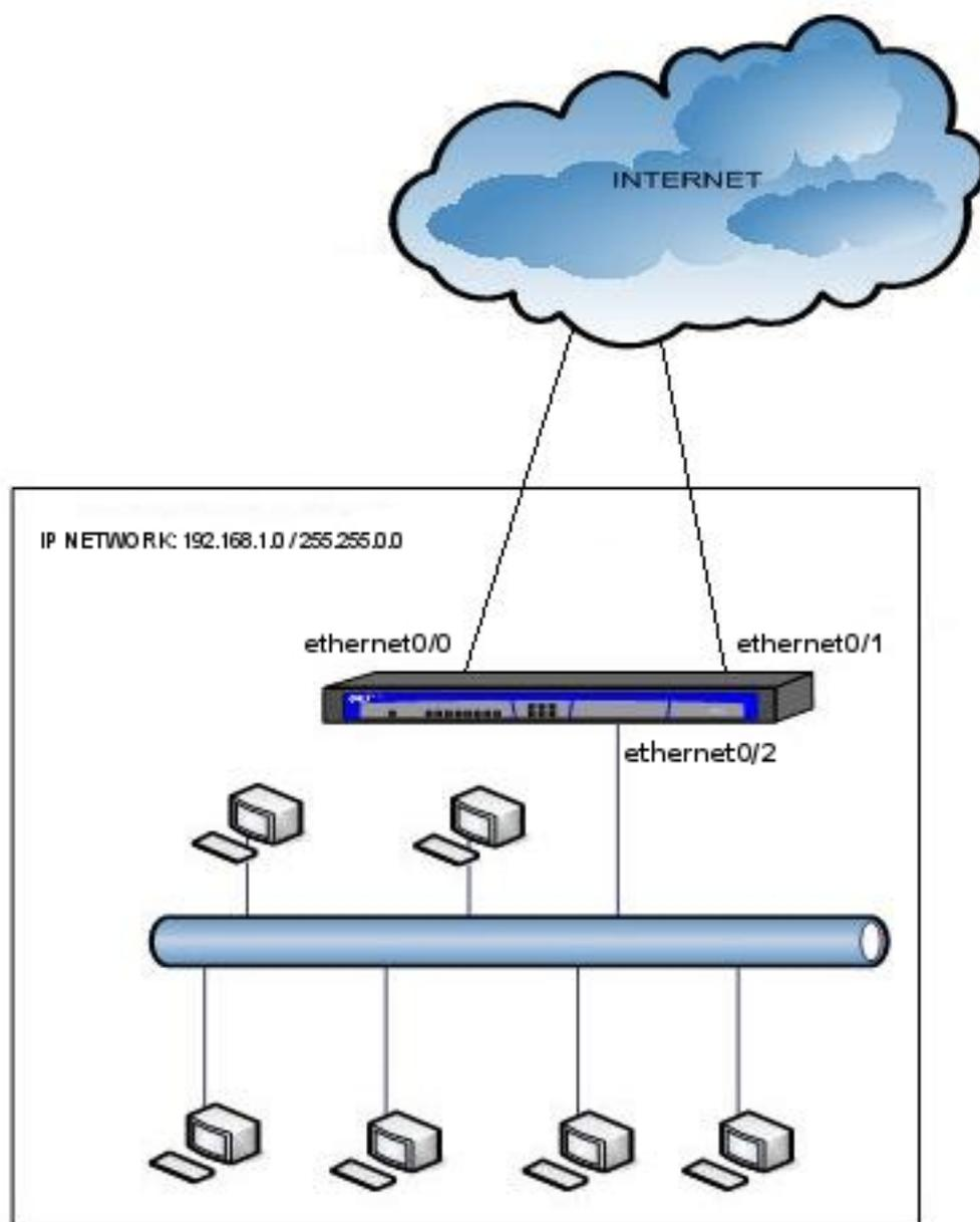
Fig. 4: Reactive load balancer
