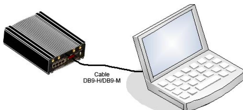
Fig. 23: **Connecting for configuration**
