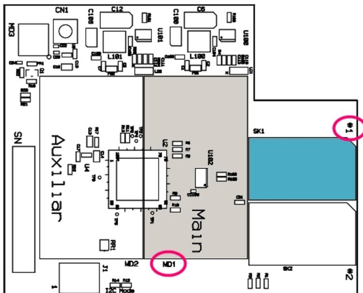
Fig. 19: SIM tray #1 for MD1 module (main)
