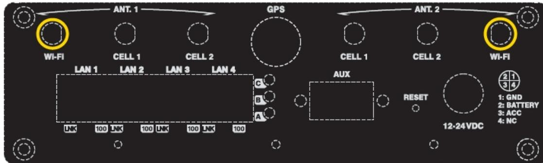
Fig. 15: ANTENNA connectors for the Wireless LAN
