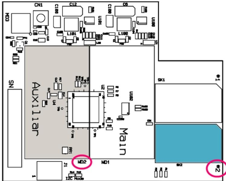
Fig. 20: SIM tray #2 for MD2 module (auxiliary)
