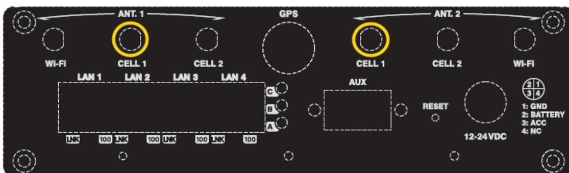
Fig. 13: Antenna connectors for WWAN 1 (with diversity)
