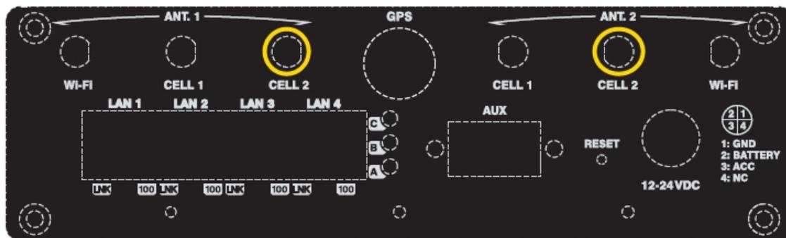
Fig. 14: Antenna connectors for WWAN 2 (with diversity)
