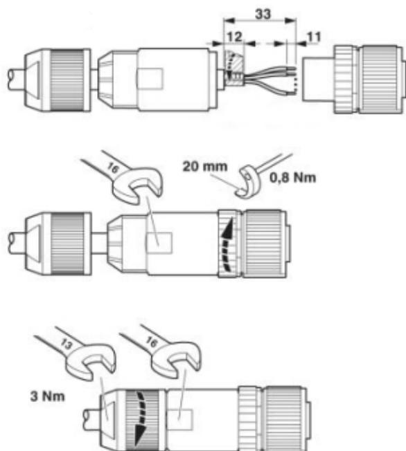
Fig. 8: Terminate the cable into the connector
