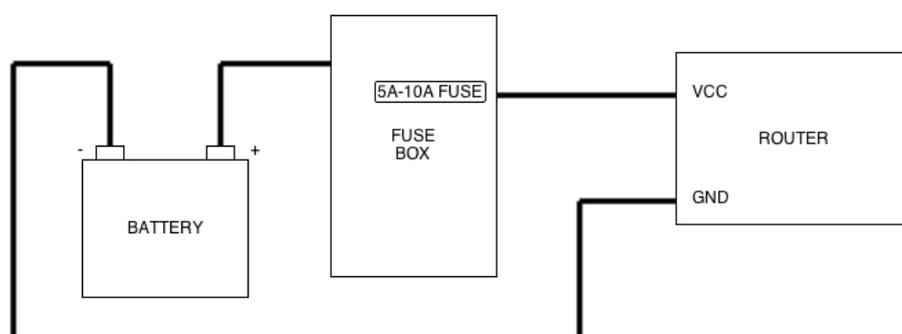
Fig. 7: Connection of Cable to vehicle power source
