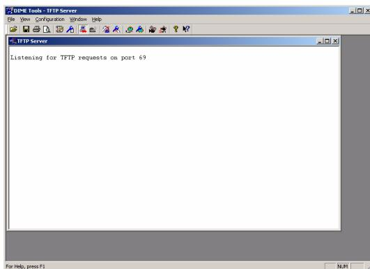
Make sure the TFTP Deamon is running. To start the TFTP server, press the following key combination in **DIME Tools**:
