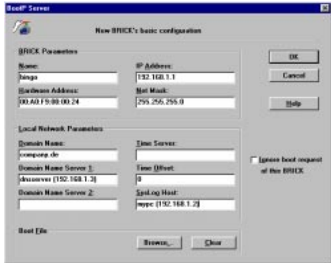
Figure 5: BootP Server – Initial BRICK Configuration
