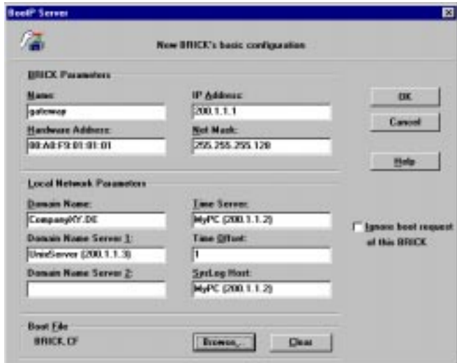
Figure 4: BootP Server – Initial BRICK Configuration
