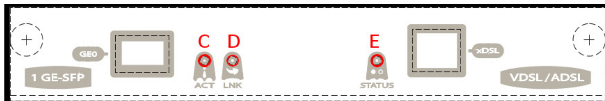
Fig. 3: TBC1-1VDSL1SFP card : LEDs.
