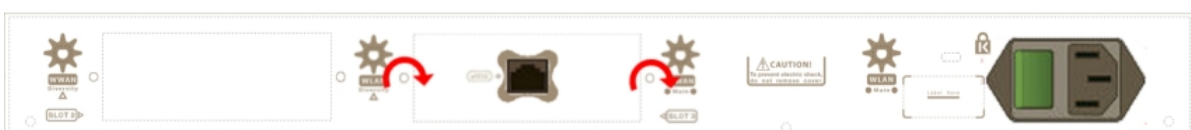
Fig. 9: Placing the expansion SLOT 3 cover
