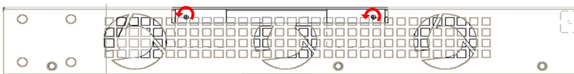
Fig. 6: Removing the screws for the top panel flap
