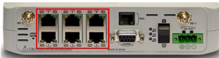
Fig. 1: Rear view of the Regesta-PRO-ER router. Switch ports.
