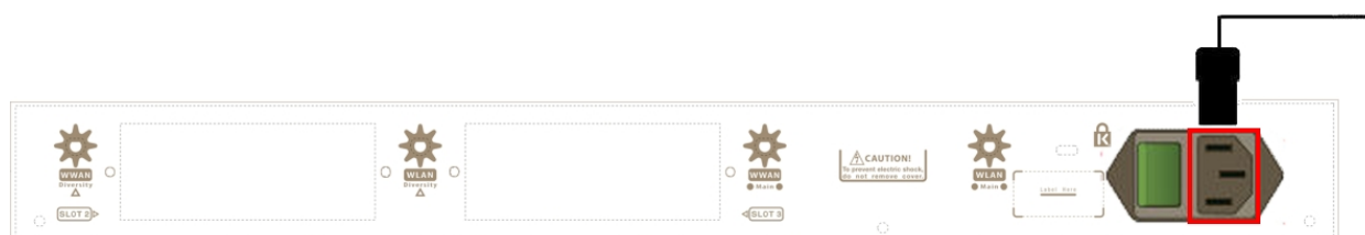
Fig. 28: Connecting the power
