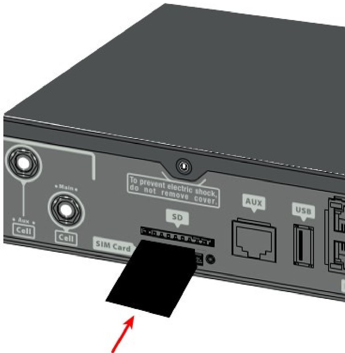
Fig. 27: Inserting SD card
