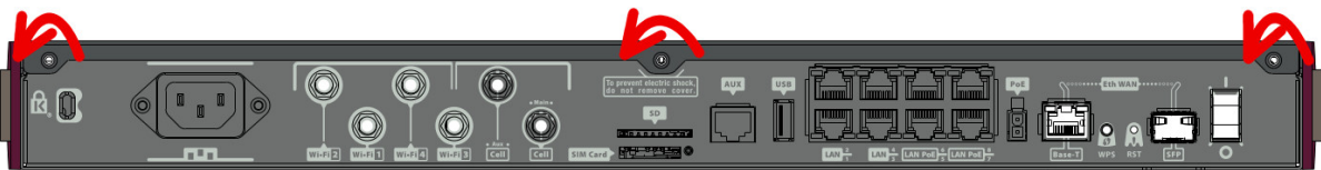
Fig. 13: Removing the screws from rear panel
