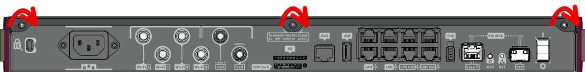
Fig. 15: Rearranging the top panel's cover screws
