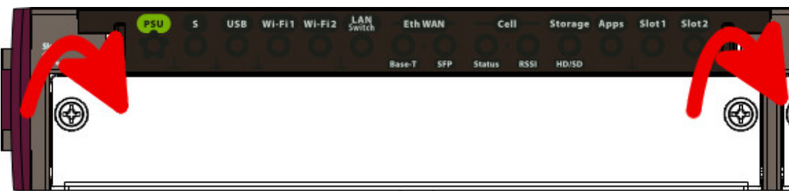
Fig. 8: Screw the tray to the front panel
