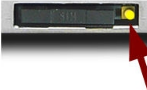
Fig. 11: Extracting the external SIM
