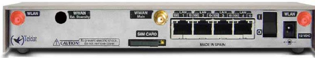
Fig. 5: Antenna connectors for the Wireless LAN
