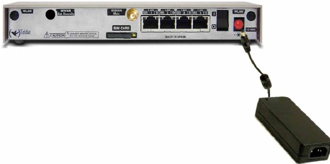
Fig. 2: Power supply connection with external source
