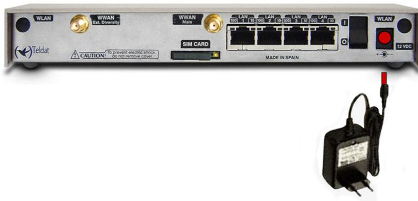
Fig. 5: Power supply connection with external source
