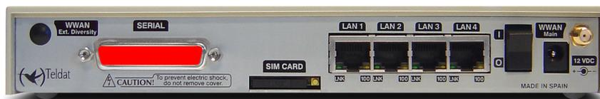
Fig. 7: SERIAL connector
