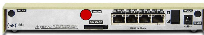
Fig. 9: Antenna connector for Wireless WAN
