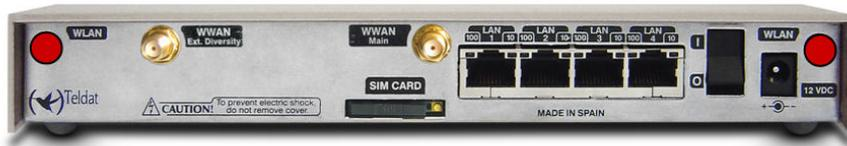
Fig. 11: Antenna connectors for the Wireless LAN
