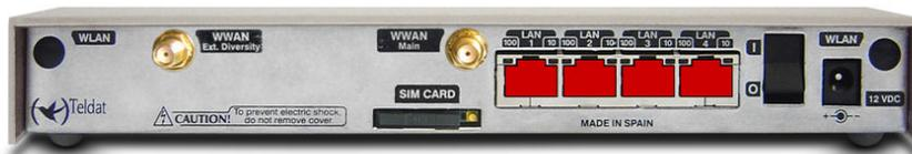
Fig. 6: LAN Switch ports (4)
