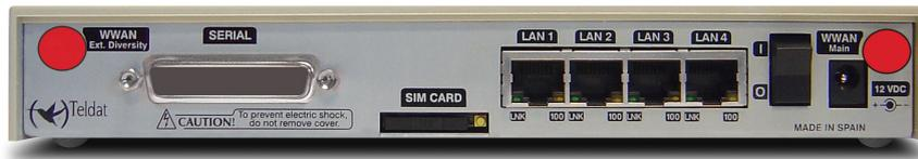
Fig. 10: Antenna connectors for Wireless WAN (with diversity)
