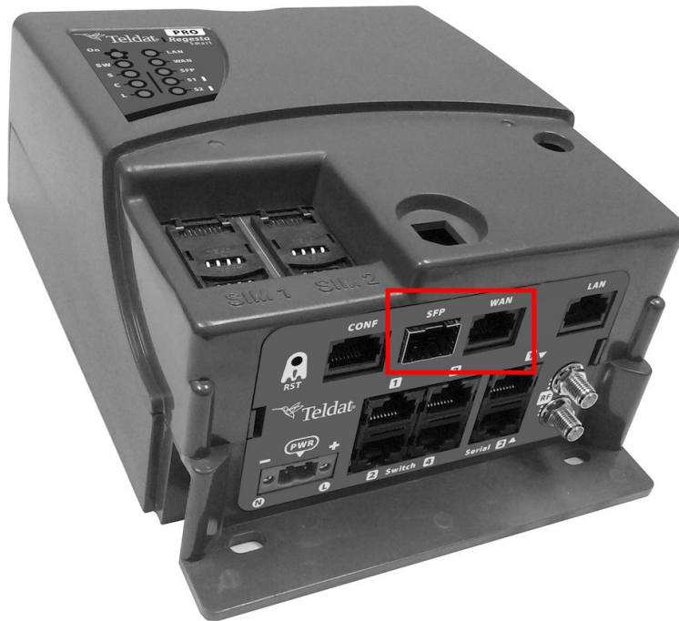
Fig. 17: WAN and SFP connectors
