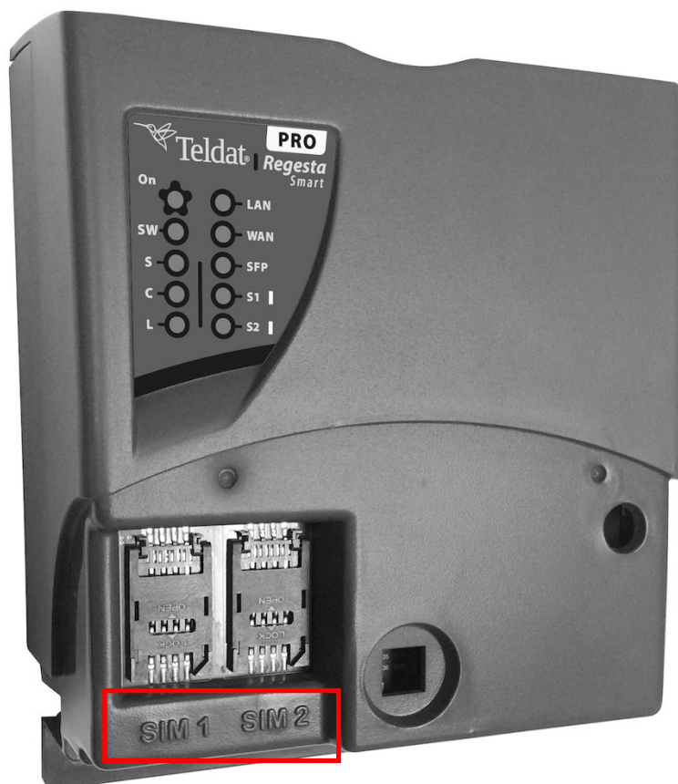
Fig. 23: Location of the SIM1 and SIM2 trays
