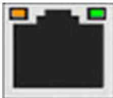
Fig. 4: WAN LEDs WAN LED indicators
