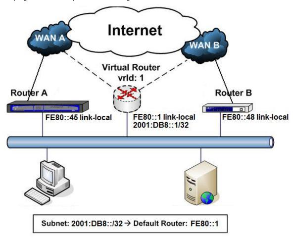
In this example, devices connected to the LAN have virtual router fe80::1 as the default router. This VRRP virtual router is defined with a primary virtual IPv6 address [fe80::1], a secondary virtual IPv6 address [2001:db8::1/32] and *vrld* identifier 1.
