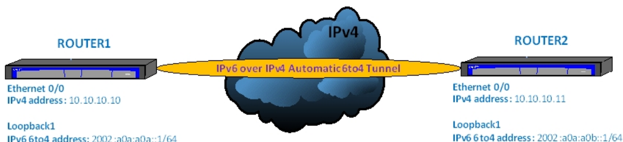
Fig. 5: Automatic 6to4 tunnel.
