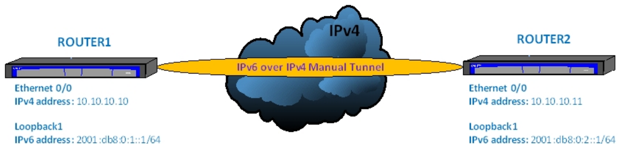
Fig. 4: IPv6 over IPv4 manual tunnel.
