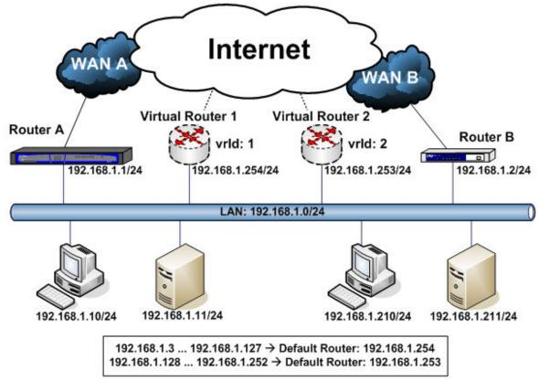
In this example, two virtual routers have been introduced: virtual router 1 (VR1: 192.168.1.254/24, vrld = 1) and virtu-
