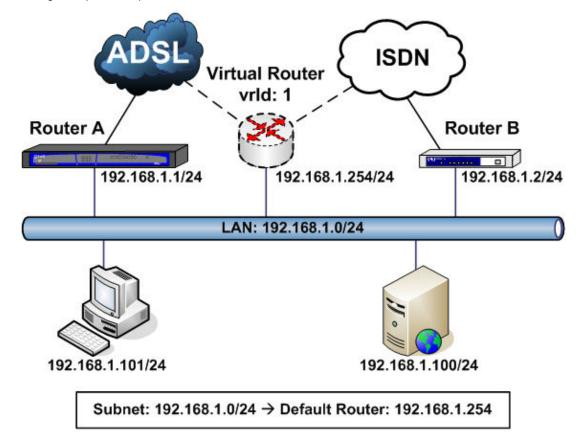
In this example, devices on subnet 192.168.1.0/24 have virtual router 192.168.1.254 as default router. Said VRRP virtual router is defined with virtual IP address 192.168.1.254 and *vrld* identifier 1.
